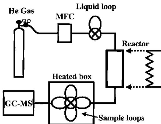
**Fig. 4** Schematic diagram of a bench-top flow reactor used for laboratory investigations of zeolite catalysis. MFC denotes mass flow controller, and GC-MS a gas chromatograph with mass spectrometric detection. The design shown delivers a pulse of liquid reactant using an automatic valve and collects multiple product gas samples (as a function of reaction time) for subsequent analysis.
