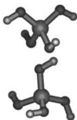
**Fig. 1**  $D_{2d}$  and  $S_4$   $Si(OH)_4$  conformations, optimized at the DF-BLYP/TNP level of approximation.
